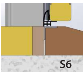
Sweep - Chiller with anti-slip Entrance Ramp
